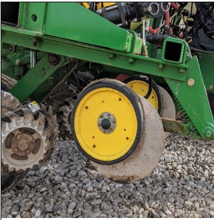
Figure 3. No-till corn planter with coulters for offset or 2x2 application provides an effective means to get N under surface residue.
