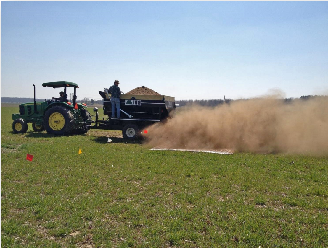
Figure 1. Spreader calibration for a poultry litter field application.
